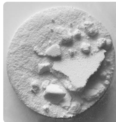
FIGURE 3. Caking of REAXIS® C154S after exposure to 40 °C and 50% RH for 24 h. Caked solids are easily broken apart after compression.
